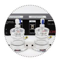
Whole Body Plethysmography - When conscious, unrestrained approaches are desired, FinePointe whole body plethysmography allows for respiratory endpoints to be obtained. This approach is often used as a quick, easy way to screen compounds, run longitudinal studies, and assess the need for further research in a more invasive model.
