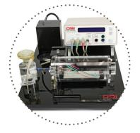
**Resistance and Compliance** - FinePointe resistance and compliance hardware helps researchers measure an animal's airflow and lung pressure. This anesthetized approach allows for direct measurement of an animal's response to a bronchoconstrictor either using an aerosol or I.V. Pulmonary fibrosis models demonstrate a decrease in compliance as a result of stiff lungs. Obstructive cystic fibrosis models affect airway resistance.
