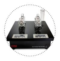
Non-Invasive Airway Mechanics - FinePointe non-invasive airway mechanics uses specially designed Allay restraint and double chamber plethysmography to monitor nasal and thoracic flow simultaneously. Aerosol administration of a bronchoconstrictor is evaluated on conscious animals deriving specific airway resistance.
