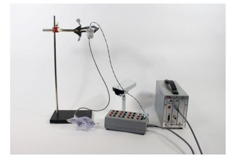
Touch proof connectors allow signals to come from the commutator to DSI's Ponemah<sup>™</sup> software using:
