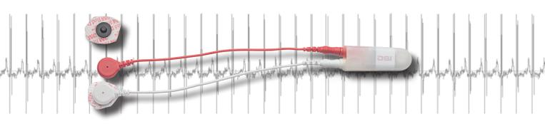
The CA-EXT is DSI's externally worn telemetry device, enabling researchers to continuously collect ECG and activity from freely moving, unrestrained rats and guinea pigs.
