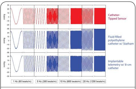
Output signals from laboratory tests of three pressure sensing systems using mechanical stimulation with a sine wave at increasing frequencies. Note that at 20 Hz, the Statham catheter had a frequency higher than the actual input.<sup>7</sup>
