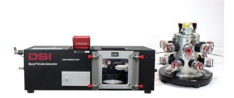
The smoke generator with a Buxco Inhalation Tower. When the exposure chambers are attached, this system will provide smoke to up to 14 subjects.
