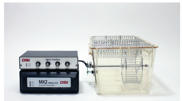
Signal Interface shown with PanLab running wheel.
