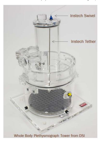
Specially designed tower caps accommodate Instech swivels and tethers; allowing researchers to conduct respiratory studies on animals when access to intravascular paths are desirable.
