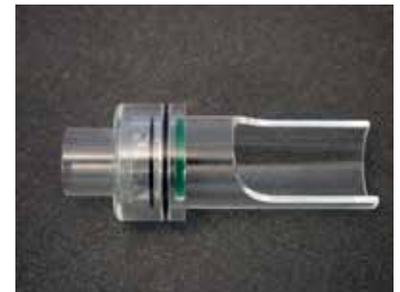
*The nose-only exposure tube for mouse. Used with the Inhalation Tower, seen on page 16.*
