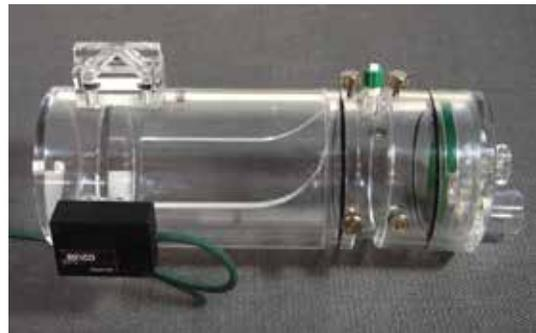
*The nose-only restraint for large rat, shown here with transducer attached.*
