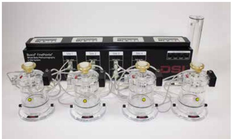
*The photo above shows a 4-site FPWBP for mouse (controller and console behind the chambers). Also available in a smaller 2-site version.*
