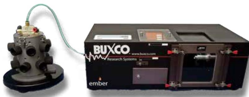
*The smoke generator with a Buxco Inhalation Tower. When the exposure chambers are attached, this system will provide smoke to up to 14 subjects.*
