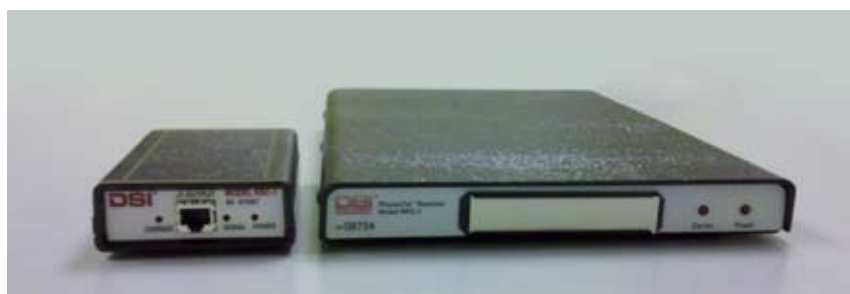
RSC-1 receiver: the smallest telemetry receiver available from DSI. Shown with RPC-1 receiver.
