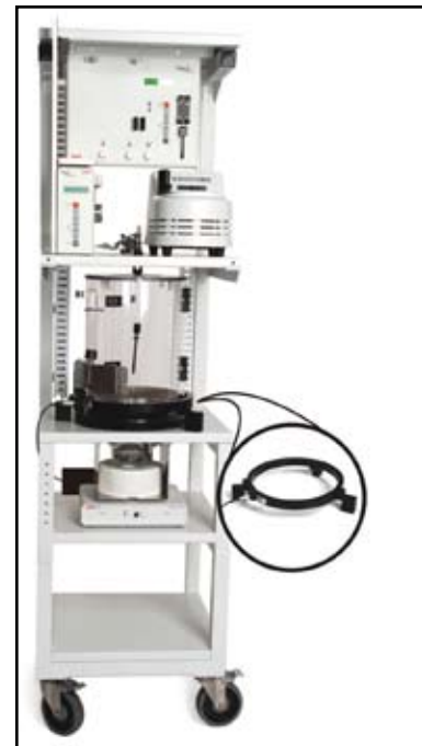
A ring antenna designed specifically for automated blood sampling applications is supported by the RSC-1 receiver.
