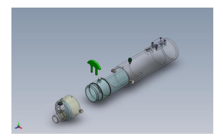
Step 3: The nose-cap was attached to the front end of the restraint tube until the Orings made a seal. Care was taken to ensure that the nose of the rat passed through the latex nose-seal to a position just beyond the whiskers (Fig 2). The rear bell of the plethysmograph was then added until the O-rings made a seal. The rats were allowed to equilibrate to the restraint for 15 min before measurements were obtained.
