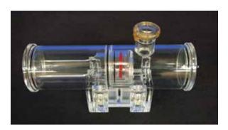
The rat plethysmograph fits onto the same footprint as the mouse plethysmograph, as does the guinea pig plethysmograph, making it possible to use only one table with several different sizes of plethysmographs.
