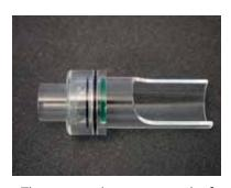
The nose-only exposure tube for mouse. Used with the Inhalation Tower, seen on page 16.
