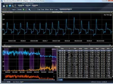
During acquisition, scrolling signal data gets recorded while simultaneously, trend graphs and tabular data are derived. All data is annotated. In FinePointe Review, you can scroll through the entire experiment.
