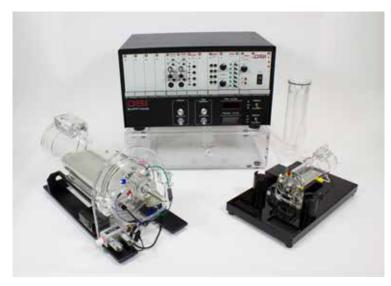
PFT controller, calibrator and chambers. The PFT system includes a control panel with pressure/vacuum reservoirs, and plethysmograph.
