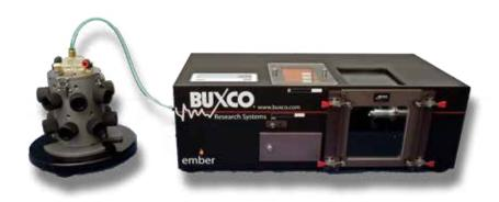
The smoke generator with a Buxco Inhalation Tower. When the exposure chambers are attached, this system will provide smoke to up to 14 subjects.
