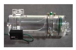
The nose-only restraint for large rat, shown here with transducer attached.
