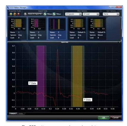
The ECG pattern manager, shown above, lets you identify example P and T waves. Click and drag to define the wave limits.
