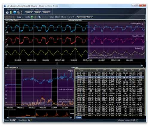
Buxco FinePointe Station software presenting data from a Buxco FinePointe NAM Site: reading thoracic, nasal, and volume signals. The bottom left of the screen displays the trend graphs for Tidal Volume and Specific Airway Resistance. The table displays the current numerical data derived from the signals presented above. Report measurement periods are highlighted in purple.
